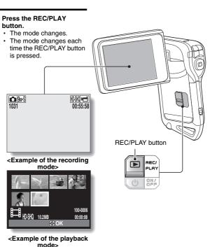
The "SIMPLE mode" comprises only those functions that are most often used and necessary to operate the camera, while the "NORMAL mode" enables full use of all the camera's many functions. Select the mode that is suitable for your purposes.
